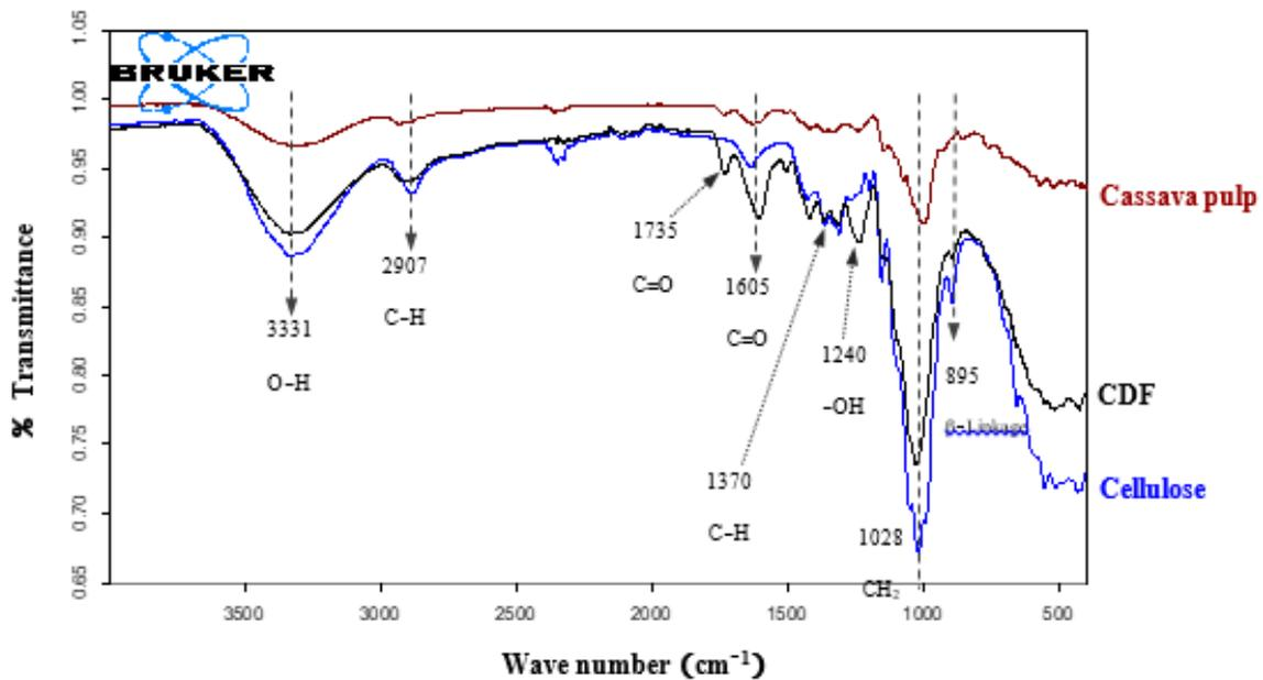
Figure 1. Fourier transform infrared spectrum of cassava pulp, dietary fiber from cassava pulp (CDF) and commercial cellulose.
